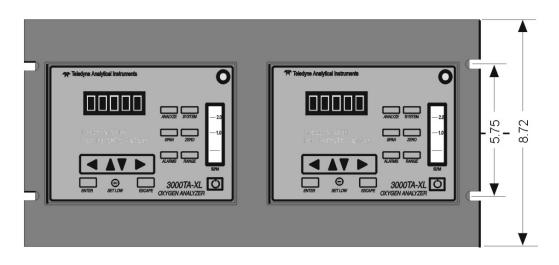
Figure A-1: Single and Dual 19" Rack Mounts (dimensions in mm)
